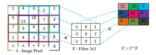
Fig. 2 Convolution Operation between Image Pixel and Filter
