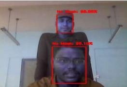
Figure 9 Screenshots of No Mask Detection with Partial Face (turned face) and Full Face using CNN
