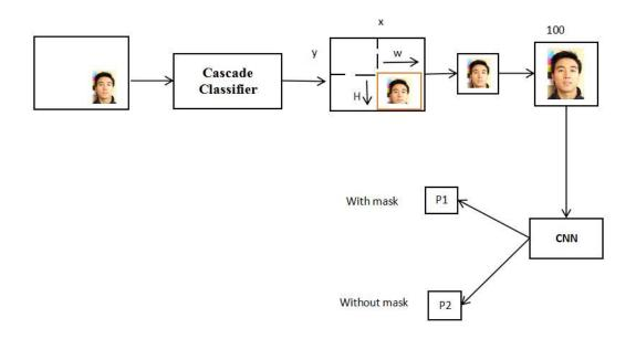
Figure 1 The block diagram of proposed Masked Face detection system
